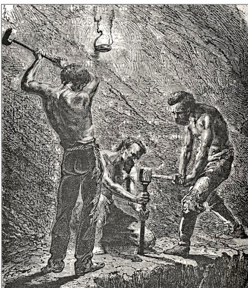
The manual boring of a hole to take an explosive charge.
