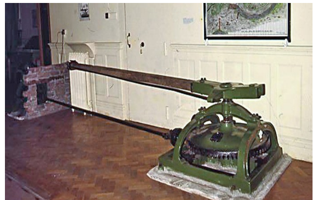
A later example of a gin with a low level drive shaft Richard Hills Collection.
