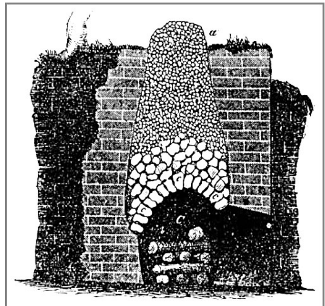
Diagram of a flare kiln showing the stone vault.
