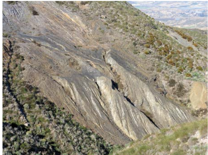
The fine grain gangue around the mine La Iberia is possibly due to the use of a cone mill.
