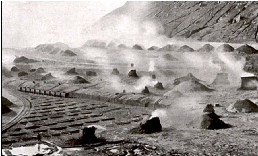
Roasting ore in the open air.
