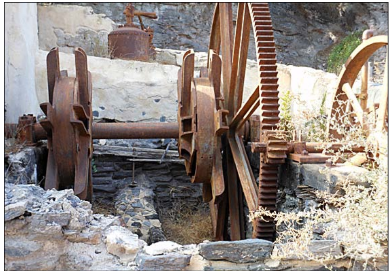
Mina Encantada's pulley sheaves and above, winding drums.
