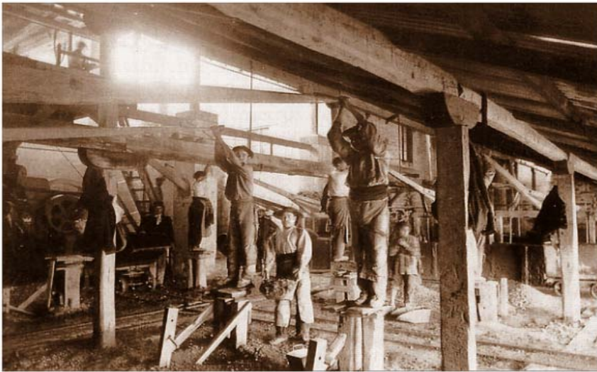
A criba cartegenera in use at a lavadero in Jaén. The pedestals and the long levers counteracted the sheer weight of the lead. T Céron.
