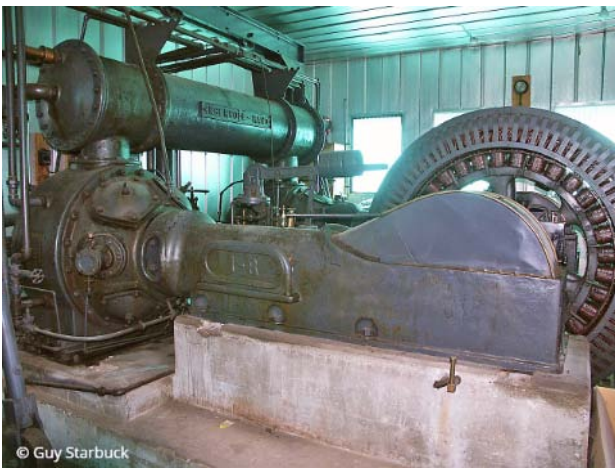
Air compressor similar to those that would have been housed in Hermosa.
