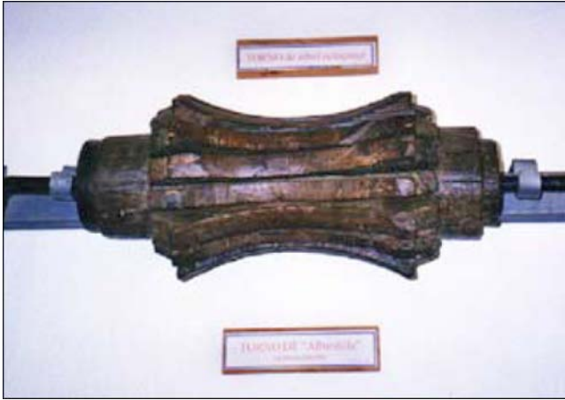
The diabolo or "saddle" drum. Dialnet-Los Castillos Mineros
