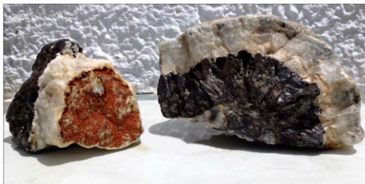
In these rock samples the white is quartz, the black is galena and the rust-coloured is pyrite.
