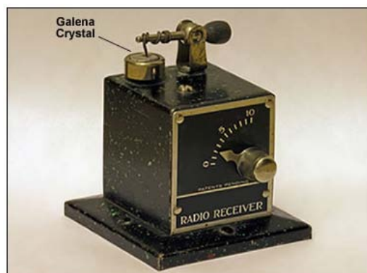
Cat's whisker radio receiver.
