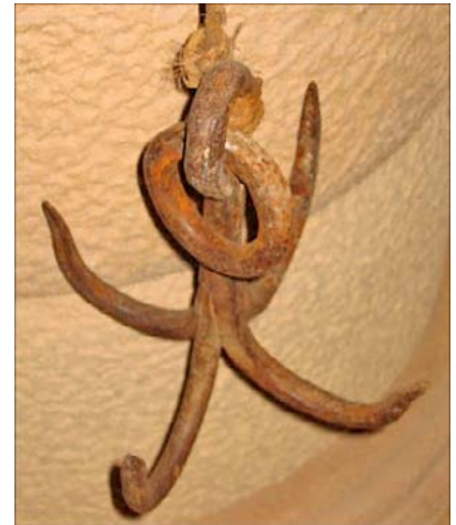
The bucket hooks often used in aljibes. The design allowed them to be tipped without spilling any water.
