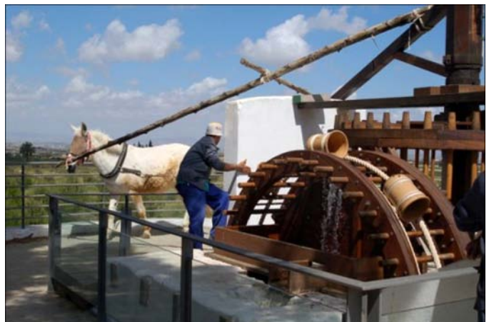
A noria in use. Note that the animal is blindfolded to prevent giddiness.
