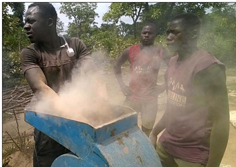
Nigerian miners grinding gold ore, with significant exposure to both lead and silica dust.
