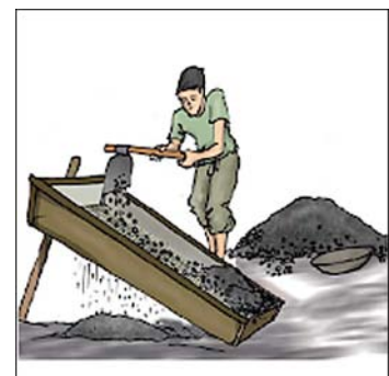
Primary screening would have either been with hand sieves (left), or with (right) ramp sieves.
